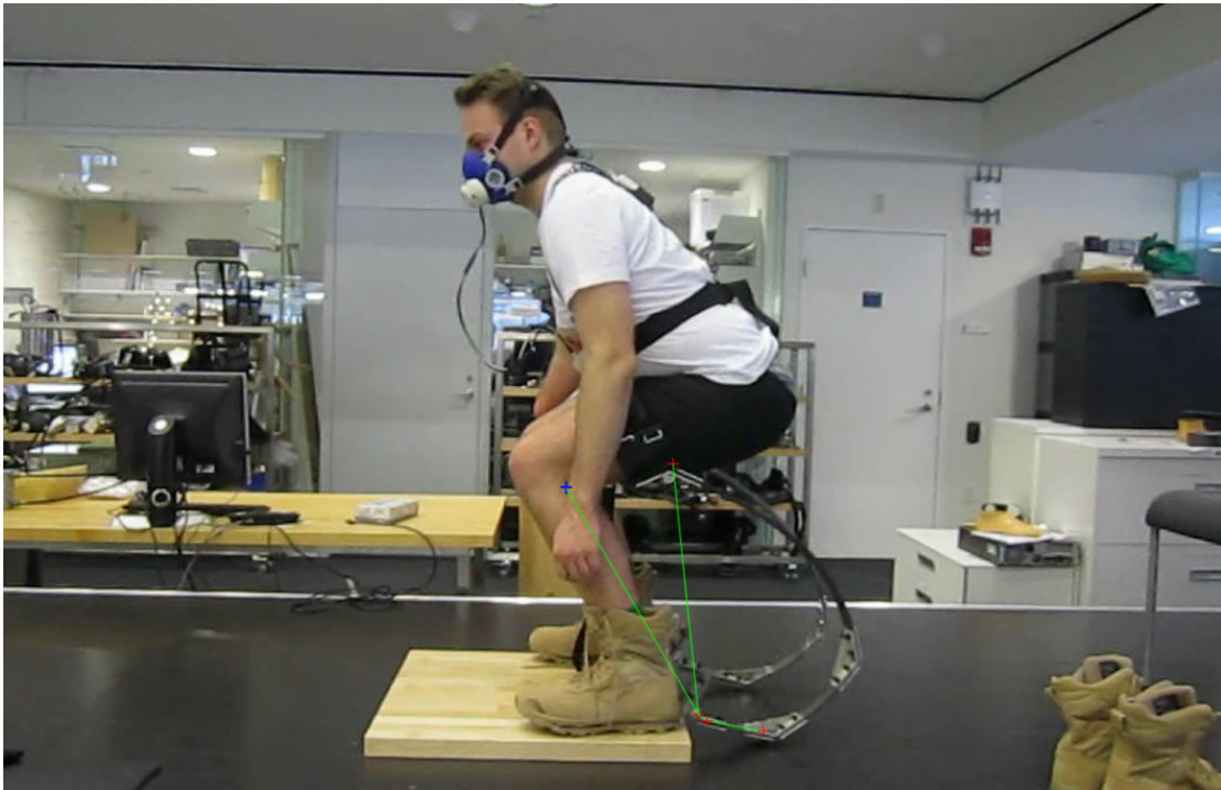
Fig. 33: Shifting the coordinate system. The two green lines indicate the distance from boot to thigh connection—the line terminating with the red '+' sign is unshifted. Blue '+' is shifted. The line in the lower right tracks the angle of the boot hinge.
