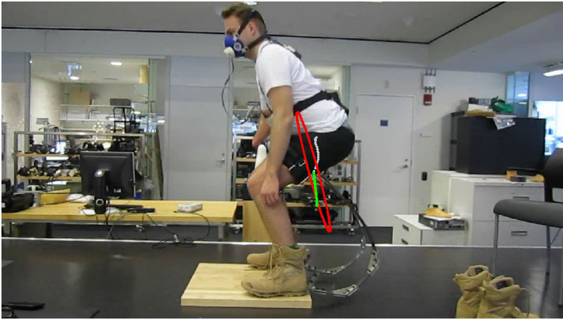
Fig. 41: Ellipse visualizations of the squat tests. The force is represented by the green vector, and the red ellipse is defined by the eigenvalues and eigenvectors of the stiffness matrices.
